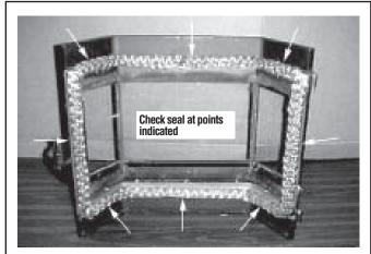
Figure 50 - Checking Door Seal
